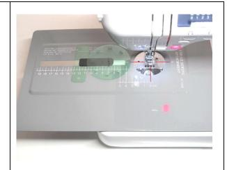
Use the plastic rectangle to place the black slide with pin. Push the rectangle under the black slide. Near the pin you can read the size of the circle.
